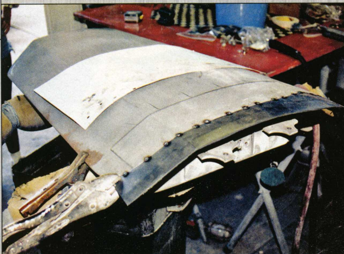
Another sight familiar to Triumph owners, the doors are the only steel in the body. A repair strip is being tacked on here
