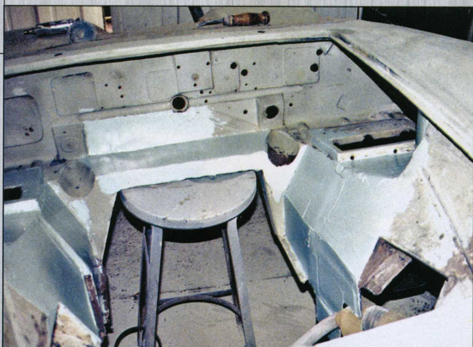
The extent of lower body fiberglass repair is visible in the blue sections. The factory bonded and riveted it to the chassis
