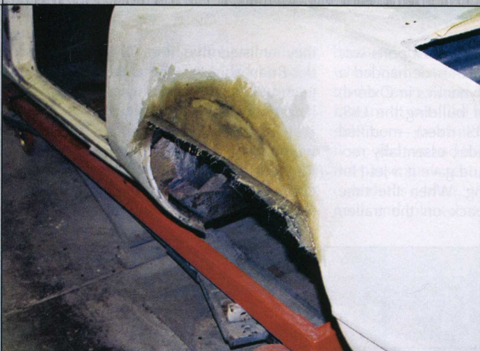
Recreating the correct wheel arches was challenging; laying up fiberglass on Scotchblok Gold paper allowed careful positioning
