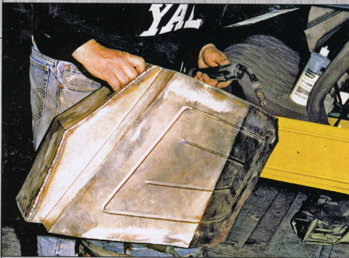
Constructing the new fuel tank. Ted Olenski leaves the steel free of rubberized coatings, and sprays with epoxy primer
