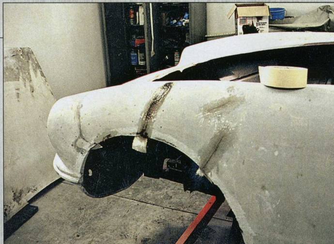
Because the front end bodywork was shattered, it was necessary to reassemble it before finish work could begin
