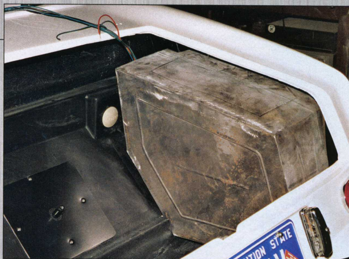
Test fitting the new gas tank, in a new location. One of Carl's reproduction silicone shock mount covers is visible just behind it
