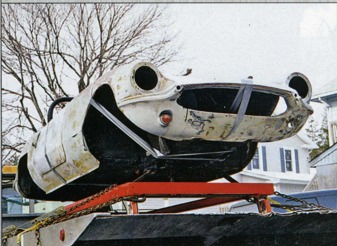
Early in the restoration, Ted tacked a lightweight transport dolly onto the frame. "It's light and easy to move, and stays out of the way"
