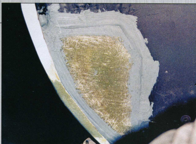
Closeup of fiberglass repair. A patch like this is glazed at the edges and feathered in with Evercoat Vette Adhesive before the gel coat
