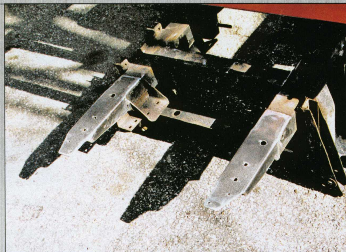
The front end of the frame, which should look familiar to Spitfire owners. The left hand rail was bent at about 15 degrees
