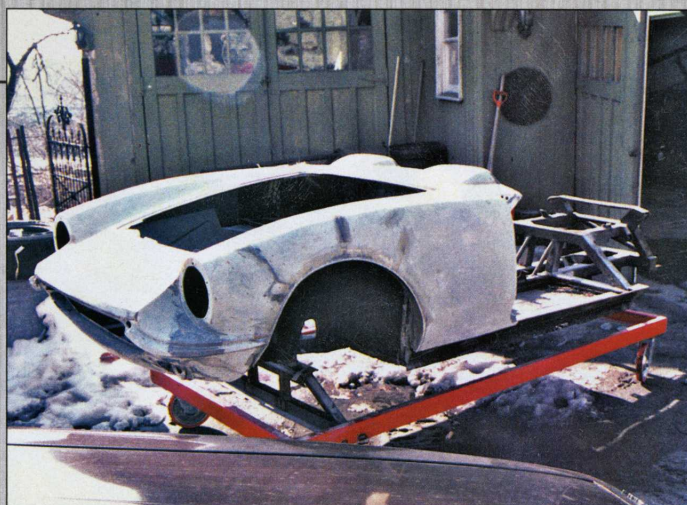
The front and rear fiberglass body sections are joined only by a fiberglass rocker section and Triumph-derived doors
