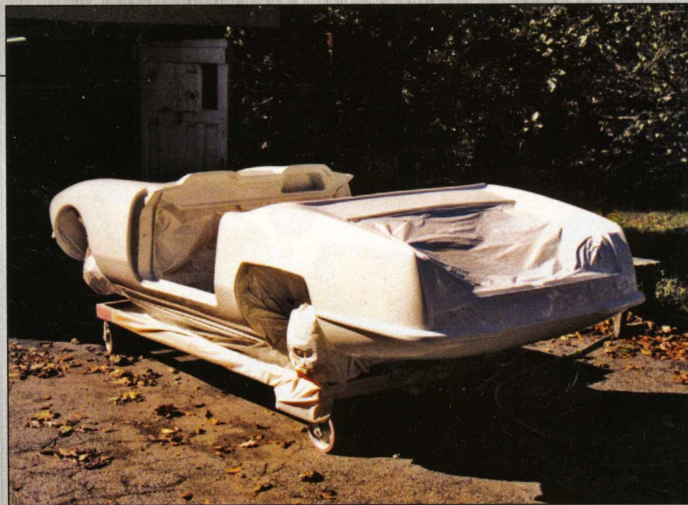
The fiberglass sections are assembled on the frame, still attached to the transport dolly. Thorough paint masking is evident
